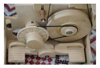
Bee - The lower left wheel is the drive wheel. The lower right wheel is the flywheel.
